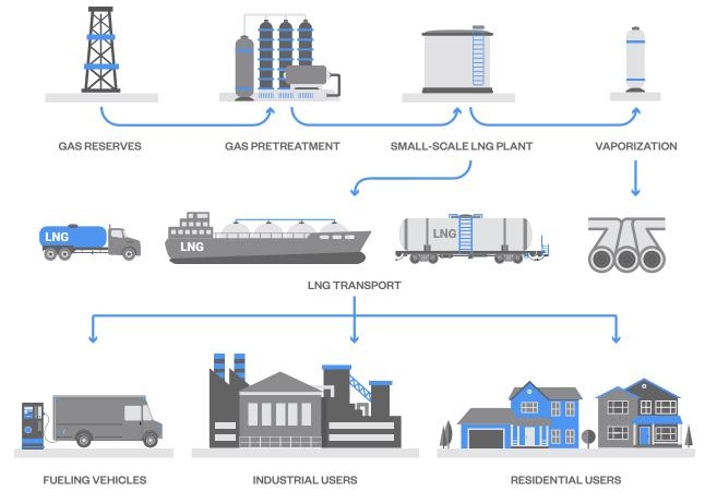
These newer applications are leading to the development of smaller scale liquefaction, storage, and regasification plants, which are far less expensive and can be built more quickly than typical baseload LNG facilities, often using modularized components.
