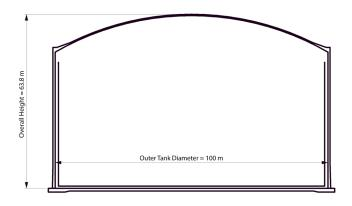
**Figure 4.** Conceptual geometry of 320 000 m<sup>3</sup> LNG tank.
