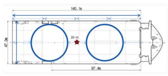
**Figure 2.** Shipping concept for two modular tanks.
