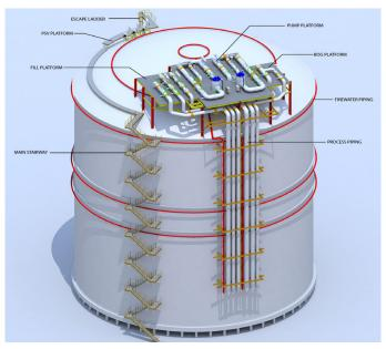
Figure 3. Rendering of modular tank concept.
