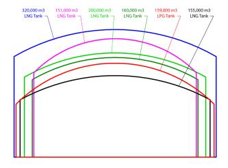
**Figure 5.** Comparative sizing of large low temperature and cryogenic tanks.
