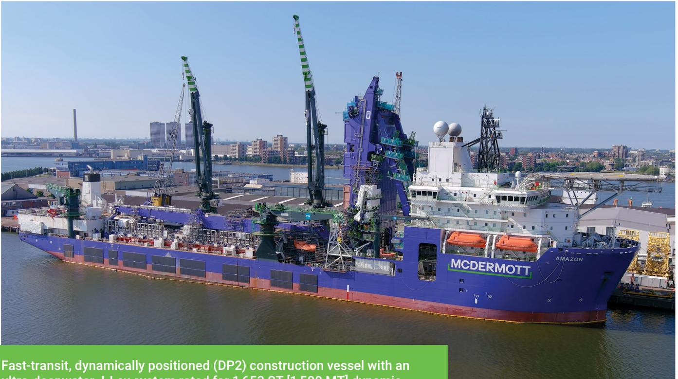
Fast-transit, dynamically positioned (DP2) construction vessel with an ultra-deepwater J-Lay system rated for 1,653 ST [1,500 MT] dynamic accompanied by two 440 ST [400 MT] Offshore Mast Cranes
