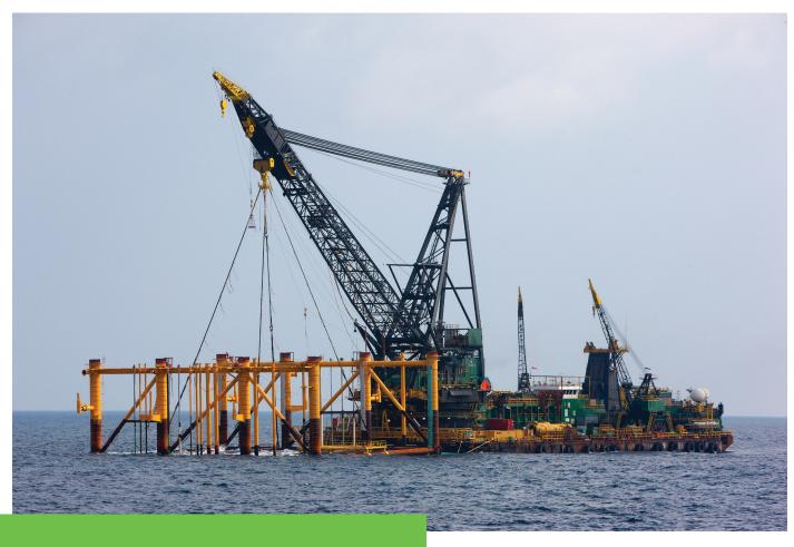
Derrick/lay barge with heavy-lift and pipelay capabilities
