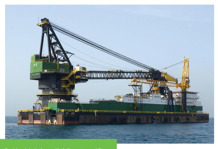
Derrick and pipelay barge with shallow water capability
