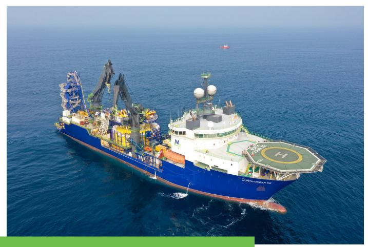
Fast-transit, dynamically positioned (DP 2) vessel with a vertical lay system for flexible product installation across a wide variety of water depths
