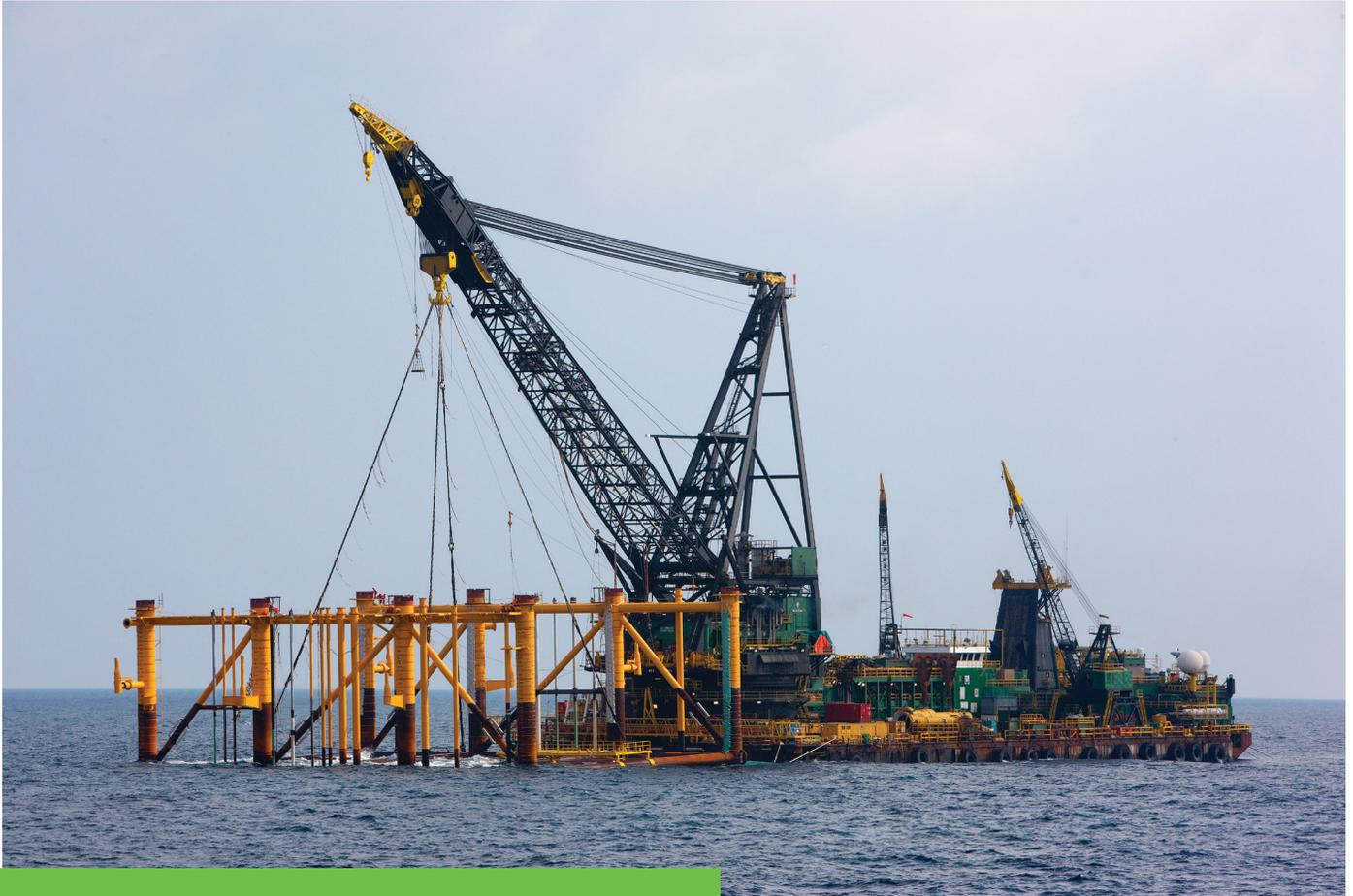
Derrick/lay barge with heavy-lift and pipelay capabilities
