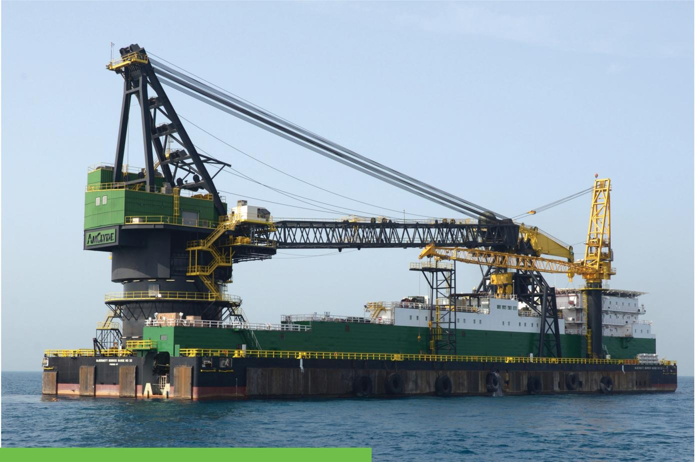
Derrick and pipelay barge with shallow water capability
